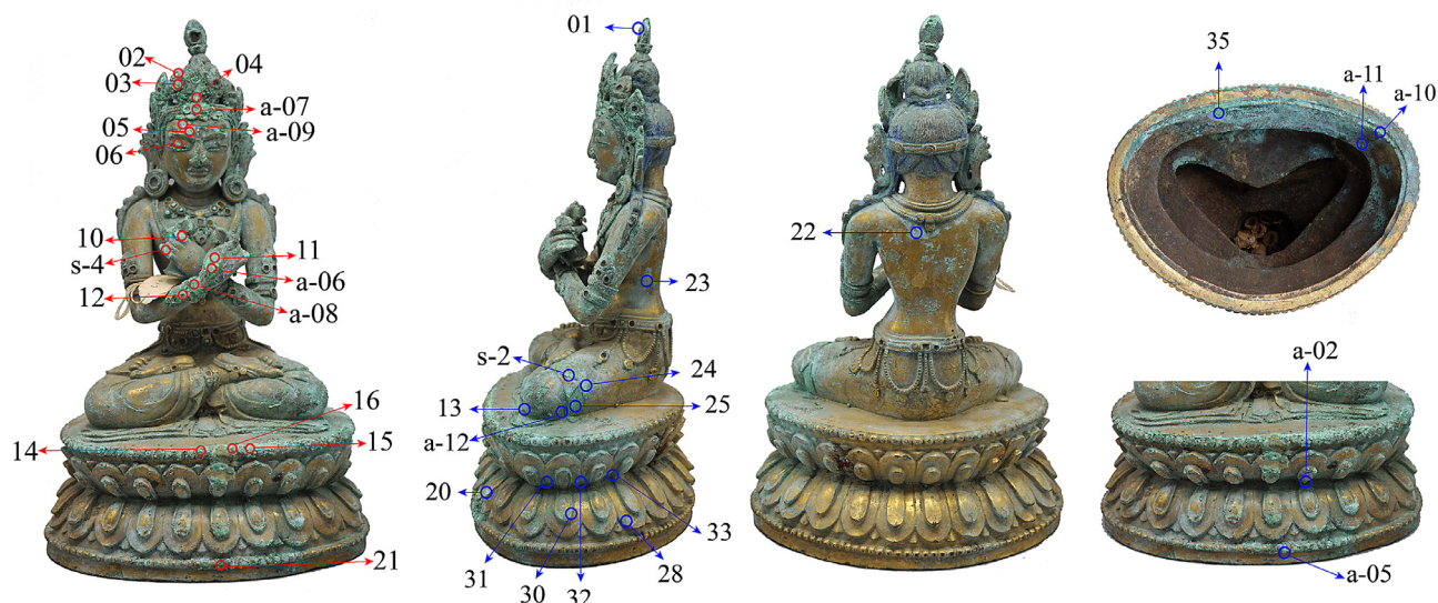
Fig. 10. The distribution “map” of the corrosion products on the gilded bronze statue “Vajrasattva Bodhisattva”. The red spots show the location of the copper trihydroxychloride and the blue spots present the location of chalconatronite.
